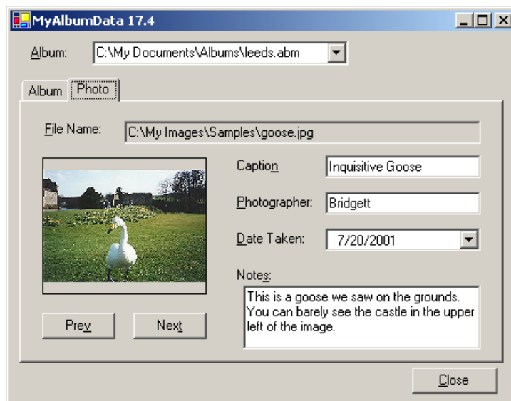
Figure 17.6 These controls on the Photo tab are bound to their corresponding values in a Photograph object.
