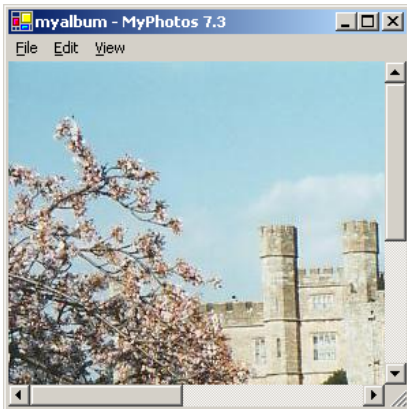
Figure 7.4 The scroll bars for the form appear automatically when the display area is larger than the client area.
